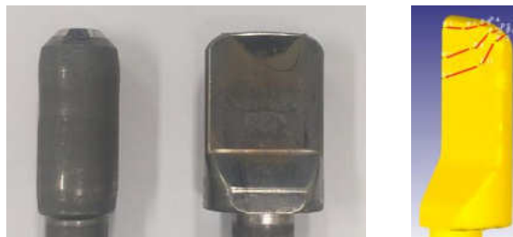
Fig.1 Development of Cut Face in the Lead Screw Forming Process
