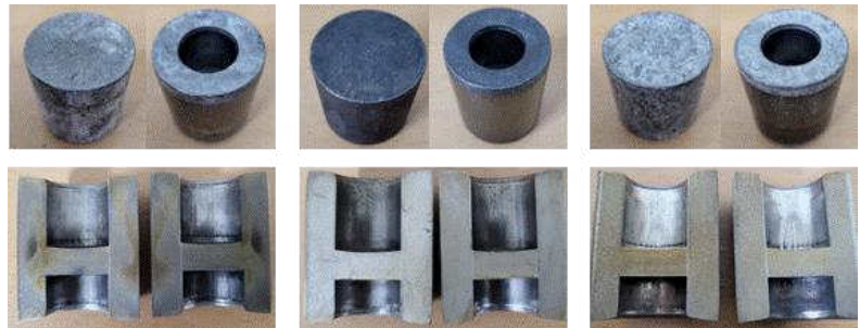
Fig. 2 Shape of specimen H-cup after friction test
